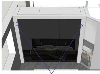
Power feeds for interanl lights coming through new stud extension and side of left and right shell
