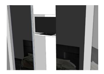
Double socket built into the middle section of the wardrobe to power TV. Joiner will need to cut hole and fix and electrician bring power to it. If the electrician is in after the joiner the joiner need to leave to make ready and leave correct cabling ready for electrician to hook up.
